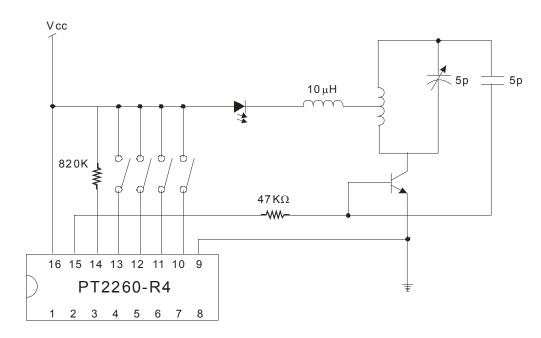
UHF Band 4-Data Transmitter Circuit is recommended.
