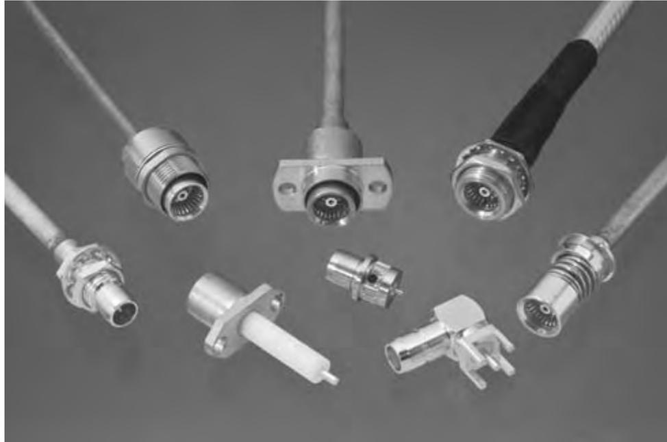
OSP miniature connectors for semi-rigid cable meet high performance requirements for microwave multiple interconnects. Standard units are available in bulkhead or panel mount designs for either direct solder or solderless compression crimp attachment. Complete tooling for both versions is located in the Tooling Section of this catalog.
