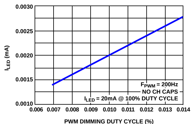
FIGURE 18. DIRECT PWM DIMMING LINEARITY AT VERY LOW DUTY CYCLE
