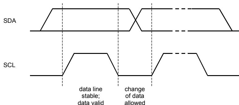
Figure 19. Bit transfer on the I<sup>2</sup>C-bus
