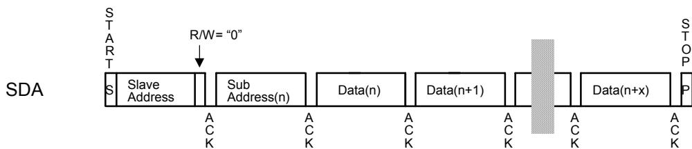
Figure 11. Data transfer sequence at the I<sup>2</sup>C-bus mode
