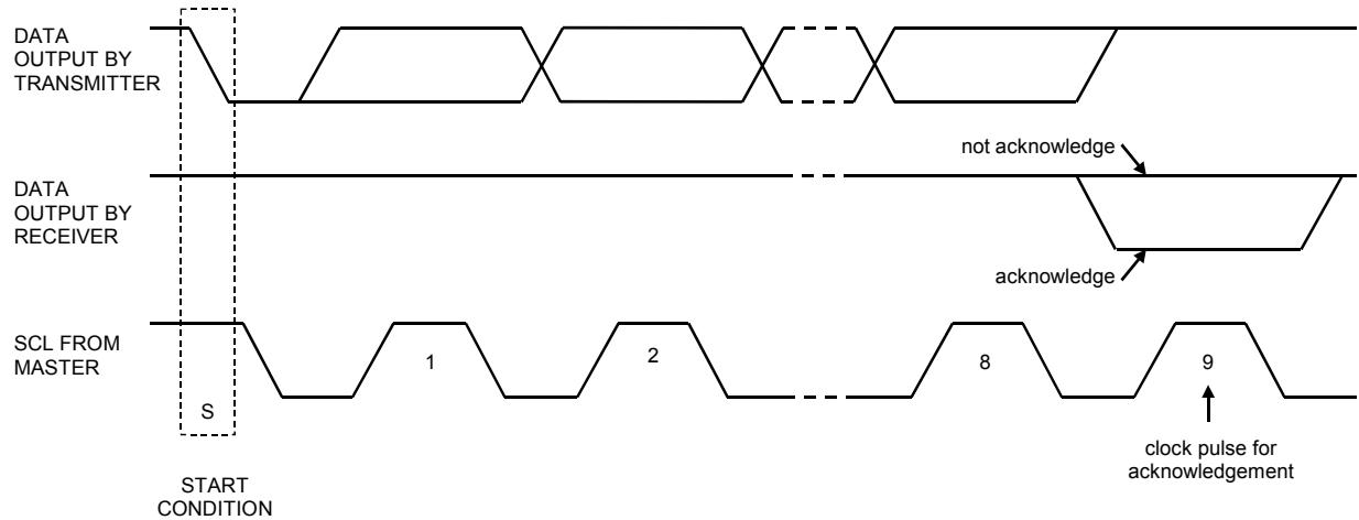
Figure 18. Acknowledge on the I<sup>2</sup>C-bus
