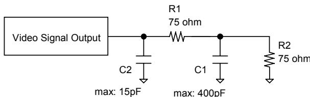
Figure 1. Load Resistance R1+R2 and Load Capacitance C1/C2.
