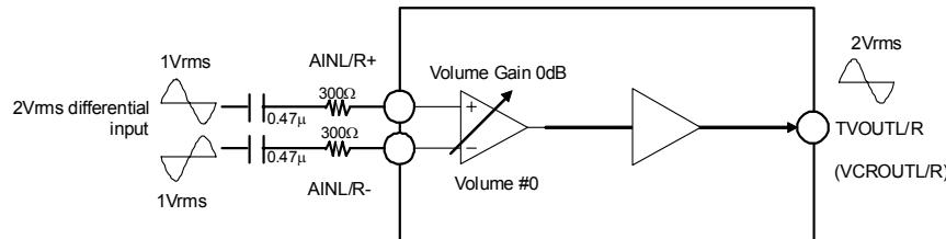
Figure 4. Volume #0(Volume Gain=0dB: default), Full Differential Stereo Input
