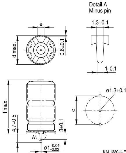
Mounting holes d = 16 mm ... 21 mm
