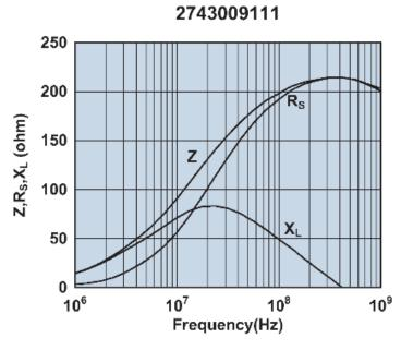
Impedance, reactance, and resistance vs. frequency.
