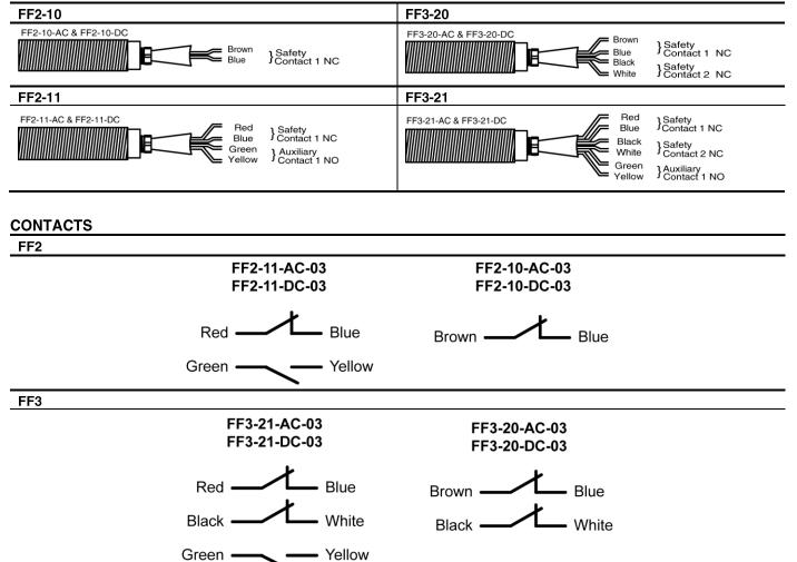
NOTE: Contact configurations show under closed condition for guard device.
