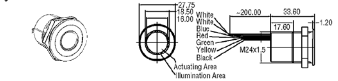
Fig. 3 Vandal-Proof Piezo Switch (Metal/Ring Illumination)
