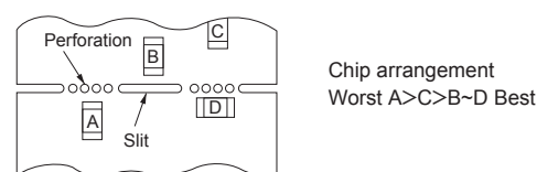
[Chip Mounting Close to Board Separation Point]
