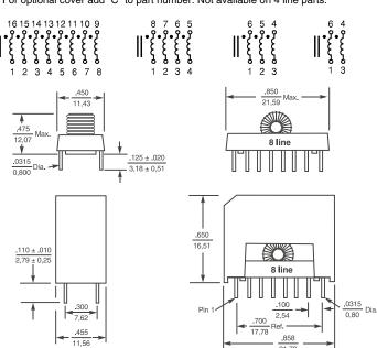
These filters are designed to virtually eliminate the problem of conducted EMI in data line applications. They provide exceptional common mode noise attenuation from 5 MHz to 300 MHz while passing signal line data frequencies below 200 MHz with minimal attenuation.
