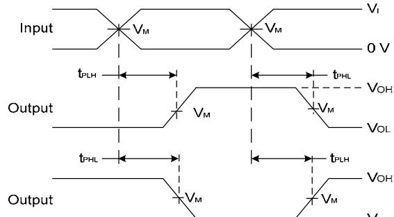
**Voltage Waveform Propagation Delay Times
