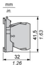
Via Integral Transformer, for BA9s Bulb
