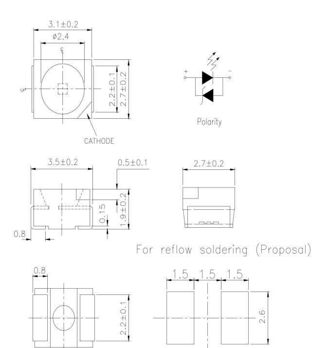
**Notes:** .All dimensions are in millimeters ,Unit = mm
