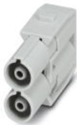
Contact insert module, number of positions: 2, power contacts: 2, control contacts: 0, Pin, Axial screw connection, 1000 V, 70 A, 6 mm<sup>2</sup> ... 25 mm<sup>2</sup>, application: Power
