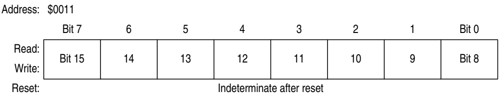
Figure 8-12. TIM Channel 0 Register High (TCH0H)
