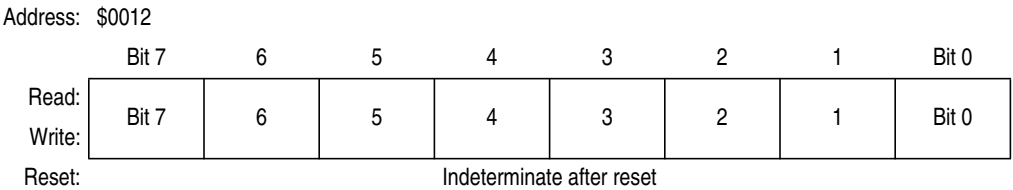
Figure 8-13. TIM Channel 0 Register Low (TCH0L)
