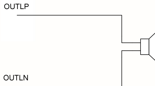
NAU8224 outputs connected to speaker without filter circuit
