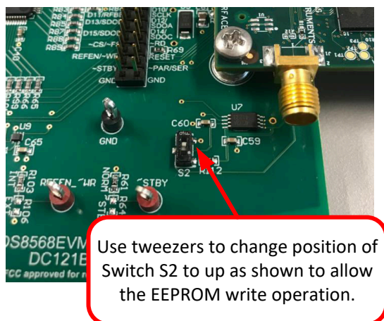
Figure 7-1. Enable EEPROM for Writing
