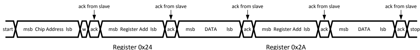
Figure 23. Multi-Byte I 2 C Command
