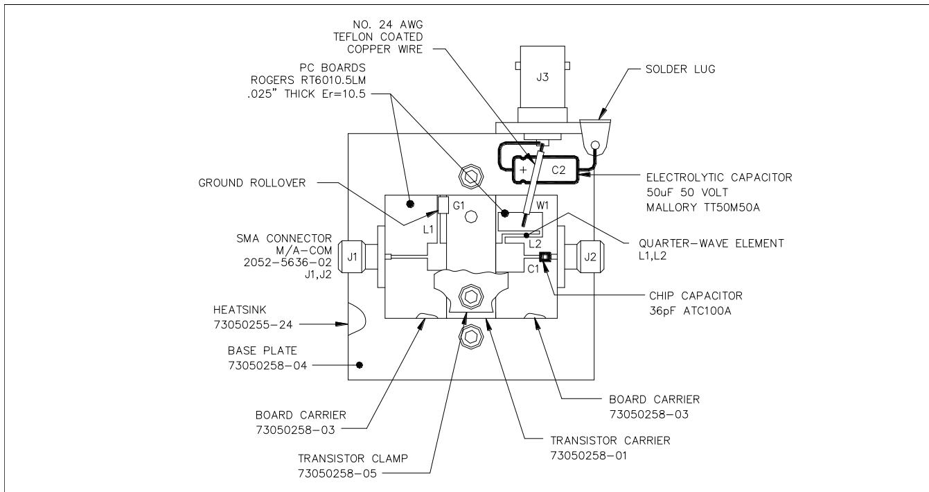
**Radar Pulsed Power Transistor
