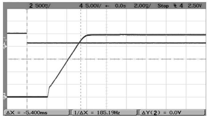
On/Off Enable Startup ( V_{IN} = 5V , V_{OUT} = 2.5V , I_{OUT} = 6A , Load=0) Trace 4=Enable, Trace2=Vout
