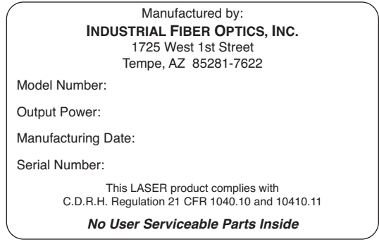
Figure 3. Laser certification and identification label.
