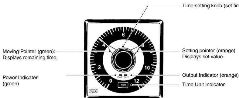
**Note:** The scale goes up to "3" with the H3AM-□-A and up to "6" with the H3AM-□-B.
