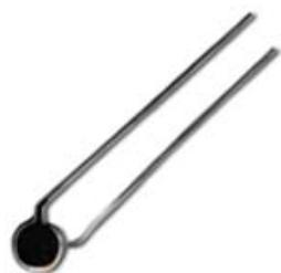
143 Series, 5,08 mm [0.2 in] disc thermistor with leads, 30,000 Ohm resistance,  $\pm 10.0\%$  tolerance, 25/85 BETA = 4261
