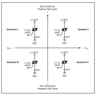
All polarities are referenced to MT1. With in–phase signals (using standard AC lines) quadrants I and III are used.
