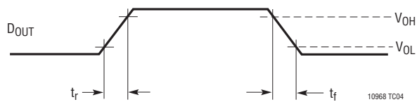
Voltage Waveforms for D_{OUT} Rise and Fall Times, t_r , t_f
