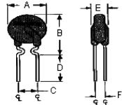
Lead Size : 24 AWG Ø0.51mm Diameter
