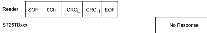
Figure 52. Reset_to_inventory frame exchange between reader and ST25TB512-AC
