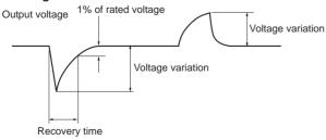
The voltage variations depend upon conditions of the input voltage and the load current.
