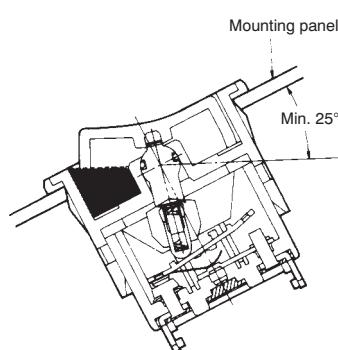
b. In case water inside the switch case may freeze, please install the switch vertically to avoid the water remain inside the switch.
