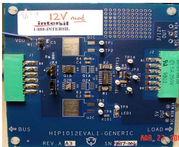
FIGURE 37. +5V AND +12V EVAL BOARD PICTURE
