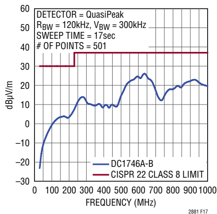
Figure 17. Low EMI Demo Board Emissions
