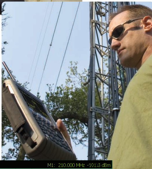
RF spectrum monitoring aided by spectrogram recording
