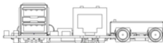
With Ethernet and 2xU.FL connectors, no USB
