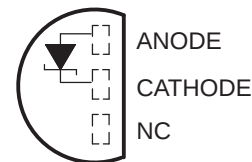
LP (TO-92/TO-226) PACKAGE (TOP VIEW)
