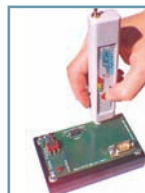
Observe how a ferrite reduces emission
