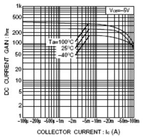
Fig.1 DC current gain vs. collector current
