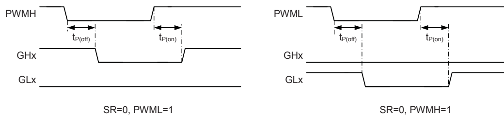
Gate Drive Timing – PWM inputs, Slow Decay, Diode Rectification
