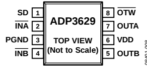
Figure 7. ADP3629 Pin Configuration
