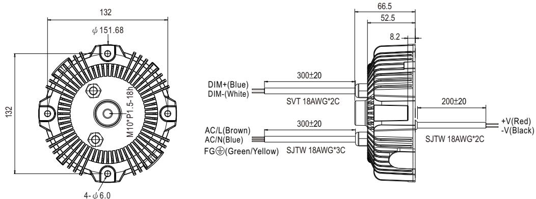
※IP67 rated. output constant current lever can be adjusted through output cable with 1-10V,PWM signal and Resistance
