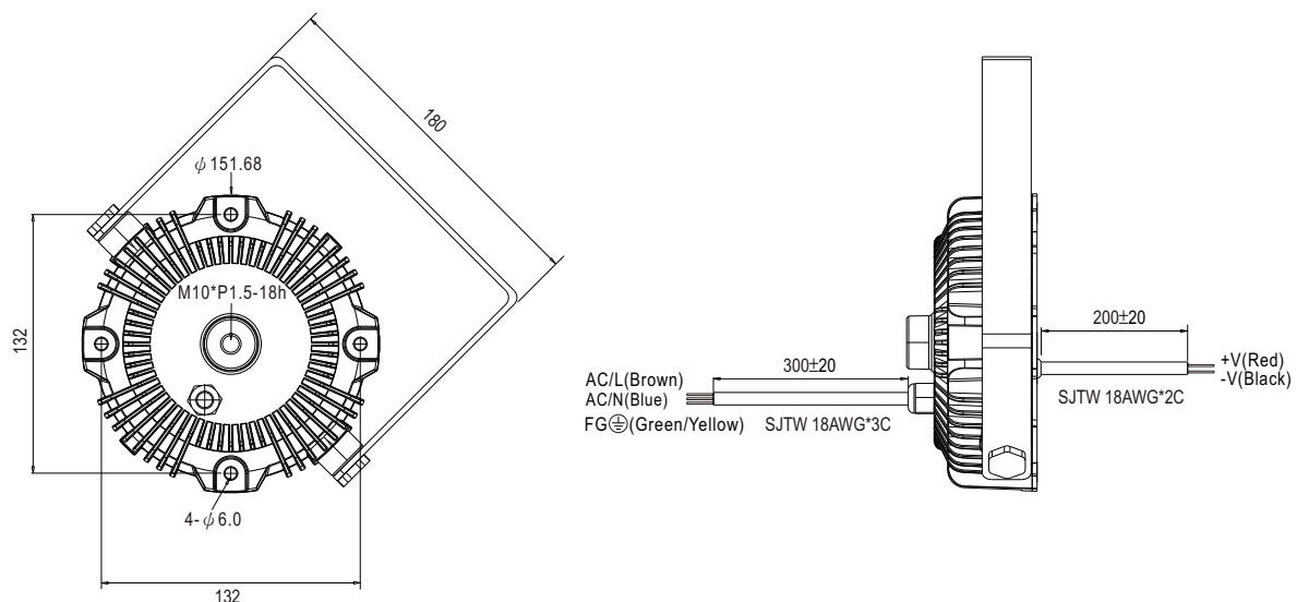
※IP67 rated. Can be fixed by steel support.
