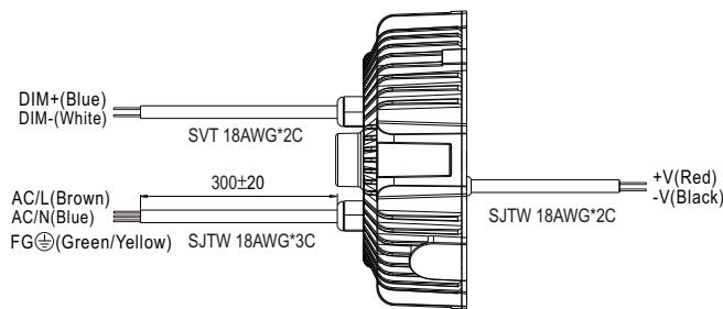
※ Built-in 3 in 1 dimming function, IP67 rated. Output constant current level can be adjusted through output cable by connecting a resistance or 1~10Vdc or 10V PWM signal between DIM+ and DIM-.
