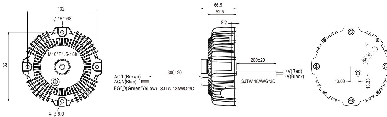
※IP65 rated. Output constant current level can be adjusted through internal potentiometer.
