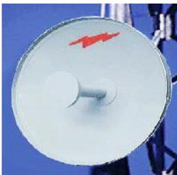
1.2 m | 4 ft Standard Parabolic Unshielded, Dual-Polarized Antenna, unpressurized, 5.250–5.850 GHz, N Female, gray antenna, molded gray radome with flash, standard pack—one-piece reflector
