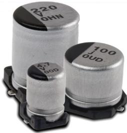
Type AVES Capacitors are rated for 1000 hours at  $105^{\circ}\text{C}$  with low impedance characteristics. They are ideal for high density PC board packaging. The Type AVES offers a low in-place-cost for a high quality performer. The vertical cylindrical cases facilitate automatic mounting and reflow soldering into the same footprint of like-rated tantalum capacitors except without the need for voltage derating. Type AVES is RoHS compliant.
