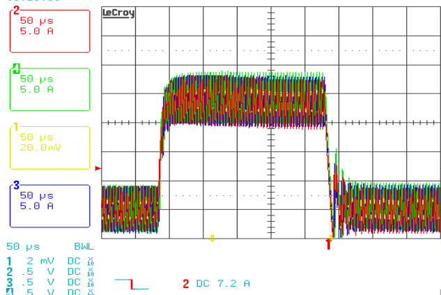
FIGURE 20. TRANSIENT LOAD 3 PHASE OPERATION - CURRENT BALANCE
