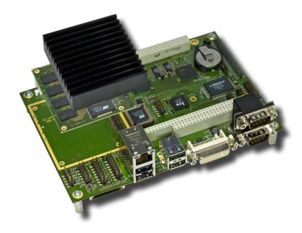
The CoreExpress Developer's kit contains all hardware and software necessary to test and evaluate the CoreExpress-ECO board.
