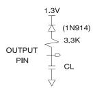
Note:  $C_L = 100 \text{ pF}$  including jig capacitance.
