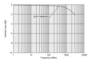
■ Differential Mode Transmission Characteristics (Typ.) **DLP11SA Series**
