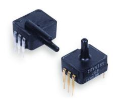
The SDX series sensors provide a very cost effective solution for pressure applications that require small size plus performance. These calibrated and temperature compensated sensors give an accurate and stable output over a 0 °C to 50 °C [32 °F to 122 °F] temperature range. This series is intended for use with non-corrosive, non-ionic working fluids such as air, dry gases and the like.
