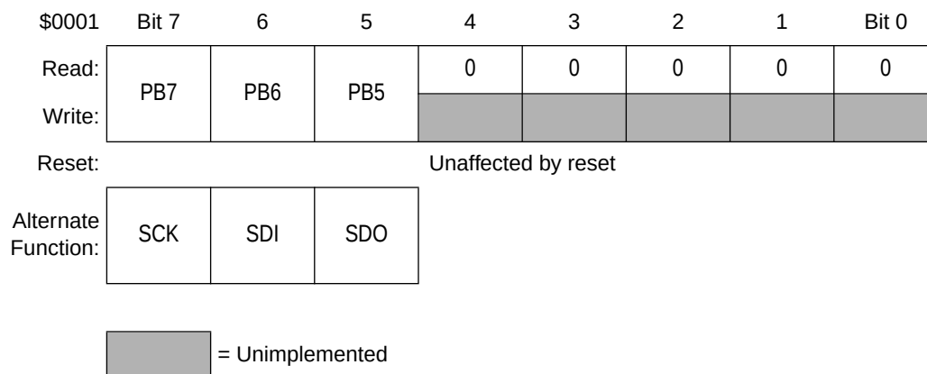
Figure 32. Port B Data Register (PORTB)
