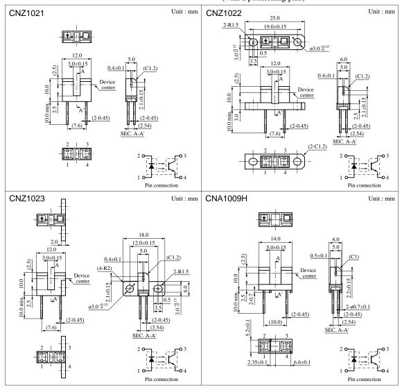
(Note) 1. Tolerance unless otherwise specified is  $\pm 0.3$ . 2. ( ) Dimension is reference.
