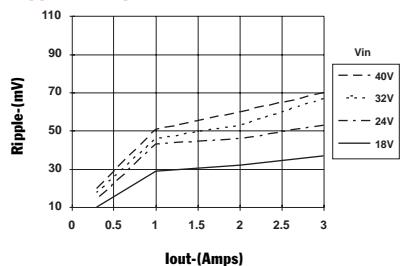
**Ripple vs Output Current**
