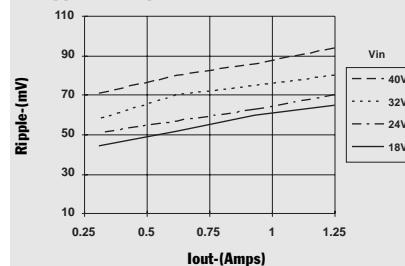
**Ripple vs Output Current**
