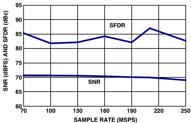
FIGURE 9. SNR AND SFDR vs f_{SAMPLE}
